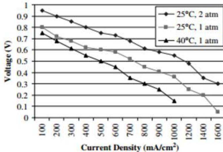
Figure 9. Polarization Curve for PEM Fuel Cells
