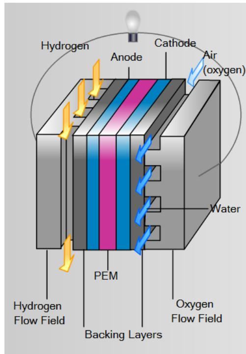
Figure 6. PEM Fuel Cell Flow Process
