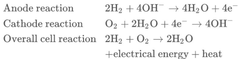
Figure 7. Fuel Cell Reaction
