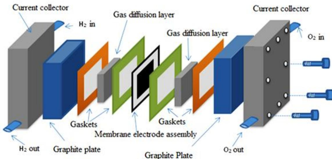
Figure 5. Assembled Fuel Cell Components
