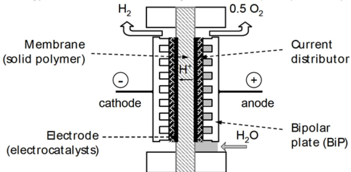
Figure 2. PEM Electrolysis
