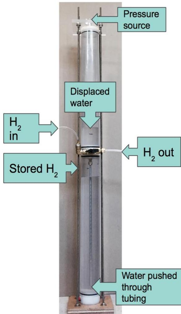
The water column stores the hydrogen created by the electrolyzer until it is ready to be consumed by the fuel cell. It operates by Hydrogen displacing water stored in the column.
