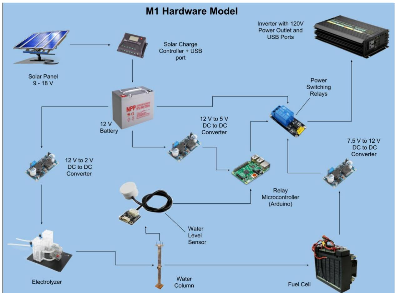
Figure 14. System diagram
